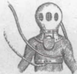
Right: Illustration of the Deane brothers' helmet and "diving dress," the first surface air supplied diving suit, 1842.
