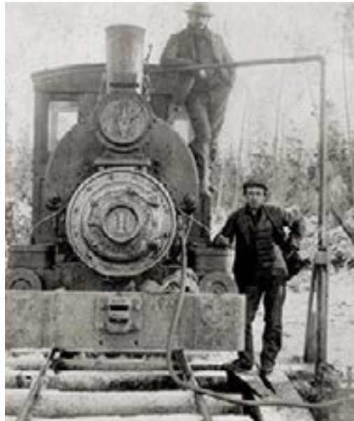
Alaska Railroad locomotive #1, built 1899 by "H.K. Porter & Co., Pittsburgh Pa." In this view, engine #1 may be working the narrow gauge route to Fairbanks, (formerly the Tanana Valley Railroad) that reached to within 39 miles of Chitina in the heart of gold mining country. This line would be upgraded to standard gauge as part of the Alaska Railroad joining Seward with Fairbanks (see Seward, this section). Porter and Co. primarily built small, narrow gauge locos that could be operated by one engineer if necessary. National Park Service.
