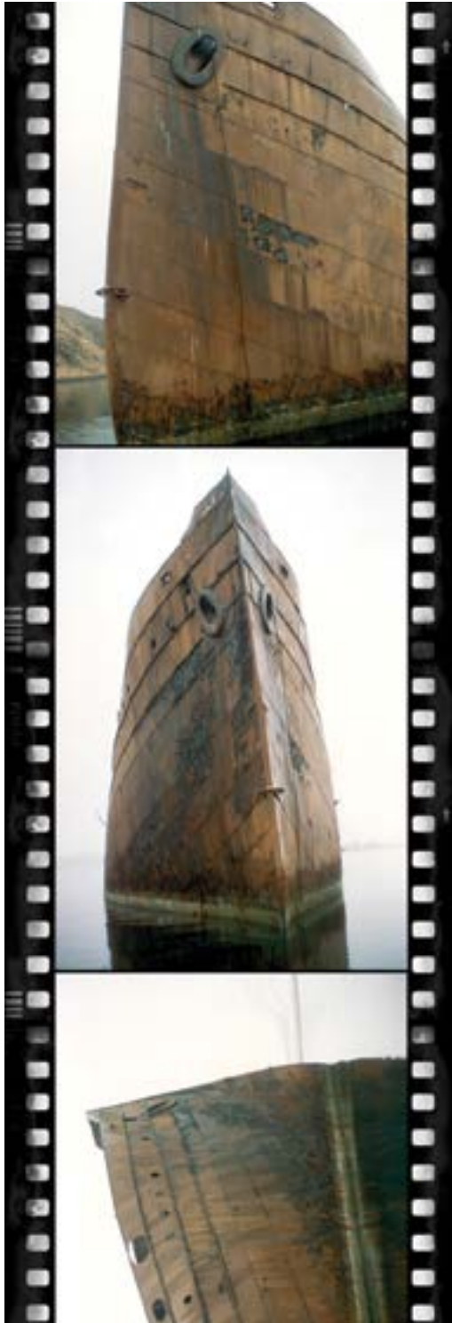
Bow of Northwestern rising 50 feet above shallow waters of Port Levashef, head of Captains Bay, May 1992. Over time, the ship's hull filled with rain water, settling the stern on the ocean floor. John H. Cloe, Historian (retired), Eleventh Air Force, Elmendorf AFB, Alaska.
