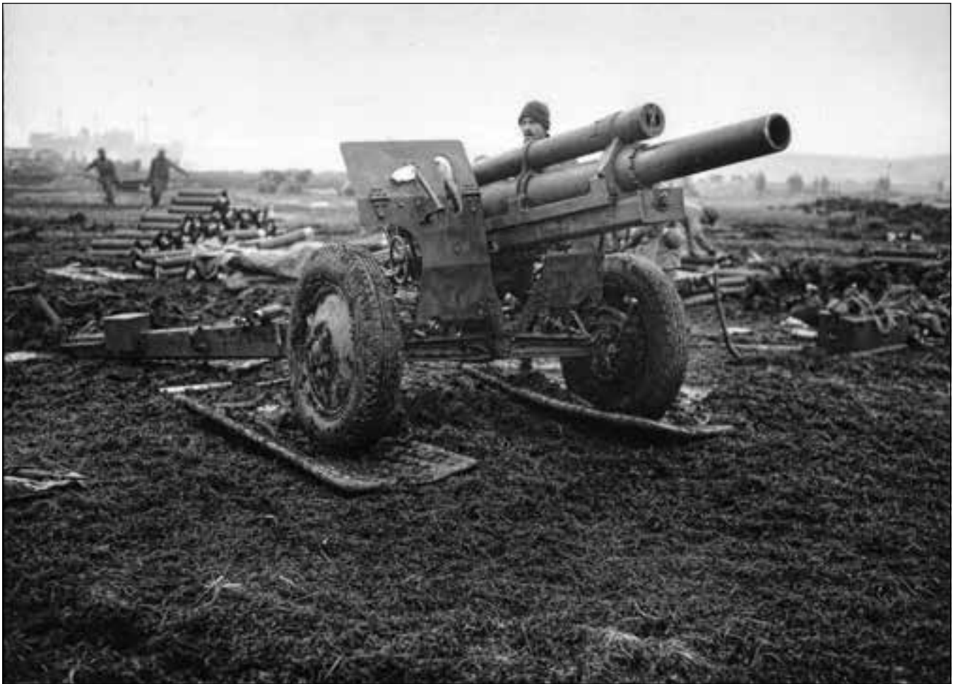
Photo IV-23: The M2A1 105-millimeter howitzer entered production in 1941 and saw service in all theaters of operation, gaining a reputation for accuracy and punch. It had an effective range of 12,270 yards and far outranged and outperformed the limited Japanese artillery capabilities on Attu. Because of the difficulty moving over the water soaked terrain on Attu, the 105s were employed from the beach area during most of the battle. This one is shown near the shoreline of Massacre Beach. (U.S. Army Signal Corps, NARA 2, RG111-148-171798)
