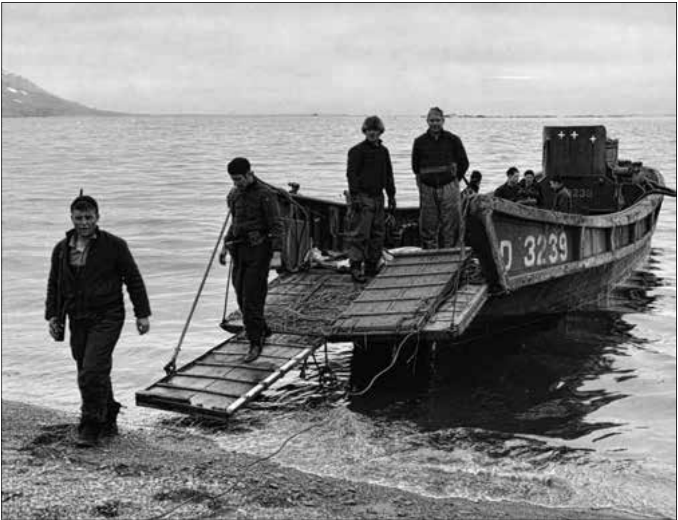
Photo IV-13: The Japanese were the first to develop a bow ramp for their landing craft, which was later incorporated into the design of the Higgins Boat. This one was among the number captured on Attu. It could carry a load of ten tons and was powered by a 80-horse power engine. (U.S. Navy, NARA 2 RG80-339-76004)
