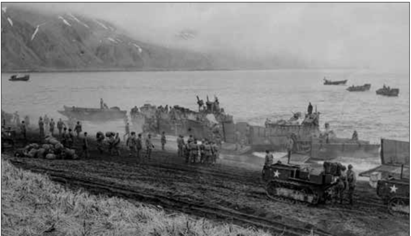
Photo V-7: The Americans used both LCVPs (landing craft, vehicle, personnel, known as Higgins boats) and the larger LCMs (landing craft mechanized) shown above on Blue Beach to land personnel and cargo. They also brought ashore small tractors which proved difficult to operate in the muskeg. (AAF, NARA 2, RG-208)
