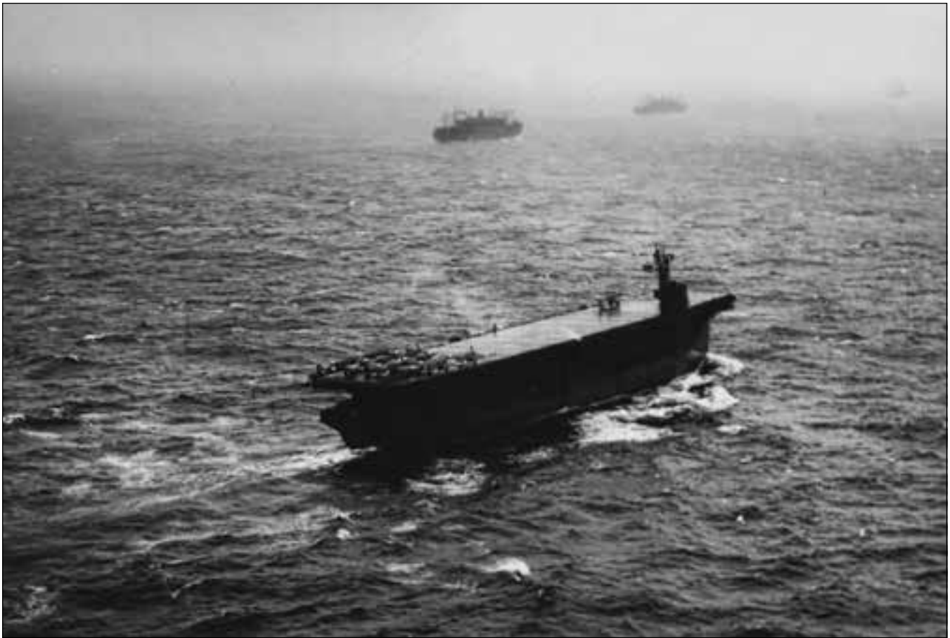
Photo IV-6: The Navy commissioned the Bogue Class Nassau (CVE-16), built on a transport hull, at the Puget Sound Naval Yard, Bremerton, Washington in August 1942. The small carrier, with a flight deck of 438-feet, was part of a fleet of so-called jeep carriers built to provide convoy escort and later used to support amphibious operations. Most were built using transport hulls. The Nassau earned the distinction of being the first escort carrier used to support an amphibious operations and the first to launch aircraft from an aircraft carrier to provide close air support for ground troops. Following the Battle of Attu, she served throughout the Pacific and well into the Cold War before being dropped from the Navy register and scrapped in 1959. (AAC, NARA 2, RG 208)
