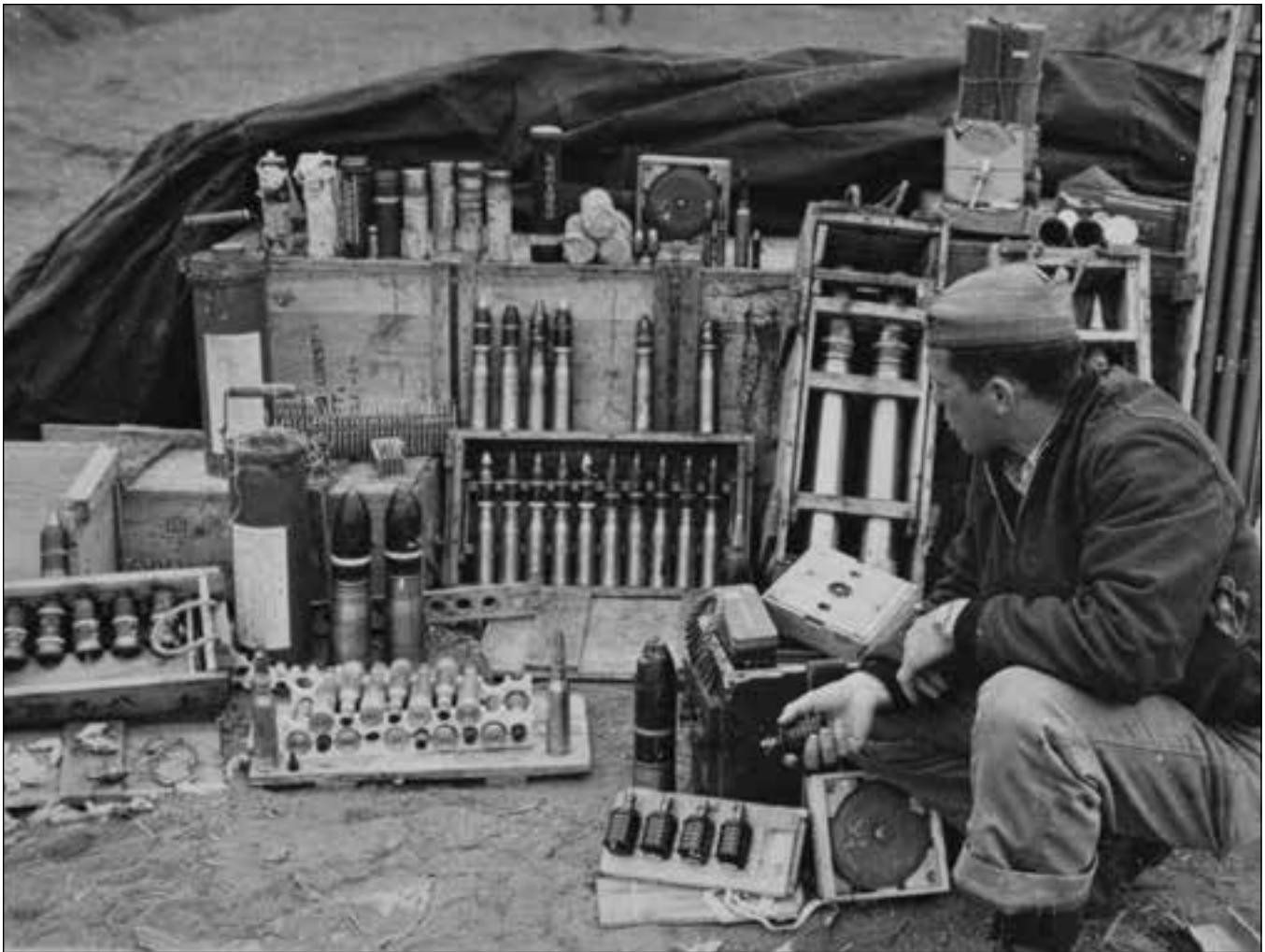
Photo V-28: In addition to stocks of food, the Americans found cases of Japanese ammunition, some of which they arranged in a display. The center section show both antitank and antipersonnel 37-millimeter rounds. The large box to the right contains two 75-millimeter dual purpose gun rounds. The three large, upright rounds are for the 75-millimeter mountain gun. Below them are 20-millimeter rounds. The Navy man holds a Type 97 hand grenade. (U.S. Navy, Pacific Region, NARA 6, RG 181)
