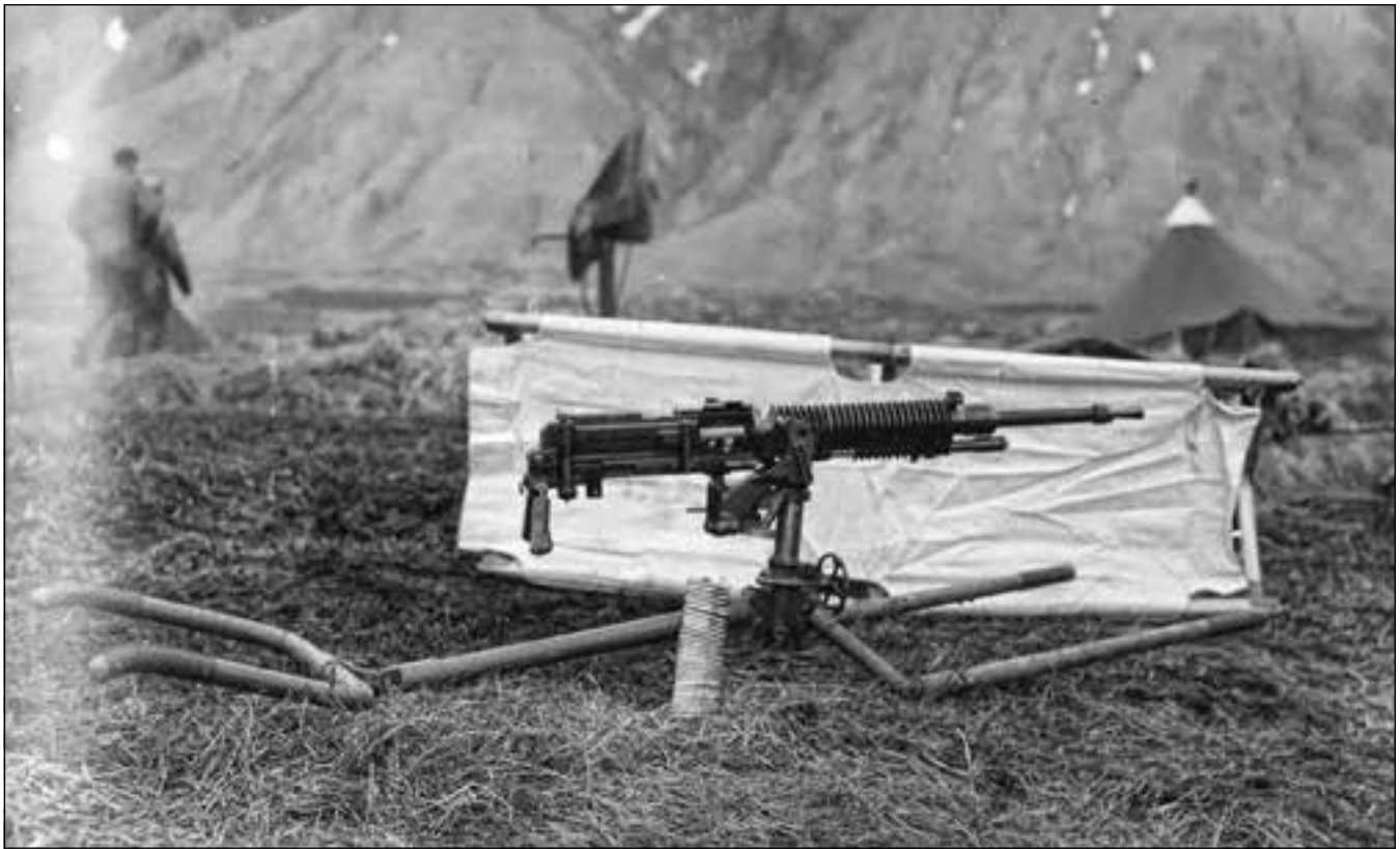
Photo IV-21: The Americans captured a large number of Arisaka heavy machineguns on Attu, one of which is shown above with its carrying handles. With tripod, the machinegun weighed 122 pounds, and unlike the Nambu light machinegun could not be easily carried in the assault. Its weight and tripod made it a steady and accurate firing platform and the slow rate of fire of 200 rounds per minute, which sounded like a woodpecker, did not overheat the barrel. (U.S. Army Signal Corps, NARA 2, RG111-169-177744)
