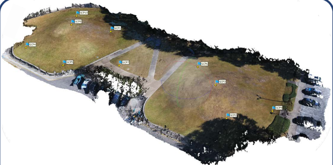
Orthorectified mosaic map of the LSU Mounds in Baton Rouge, LA. Note the flags that represent GCPs. Credit: Kory Konsoer, Louisiana State University.
