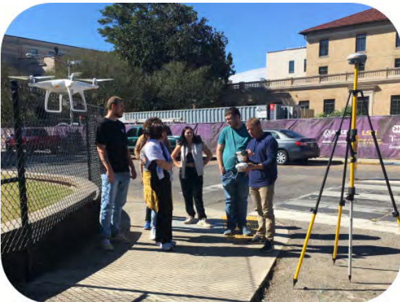
Preparing an sUAS for survey. Note the aircraft in top left corner, and GPS antenna in the right frame. Credit: Kory Konsoer, Louisiana State University.
