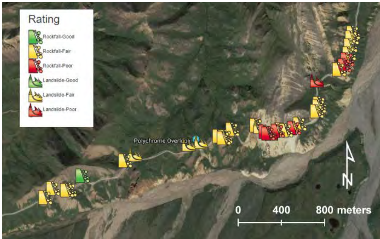
Figure 4. Annotated screen capture of the Geotechnical Asset Management Program story map from mile 44 to 46 of the Denali Park Road. On the webpage managers can click on icons for more detailed information about each entry. [Ratings are based on the frequency and severity of rockfall and landslide events.]
