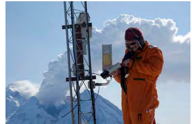
Figure 2. Cyrus Read, AVO/USGS, installing the new, zoom-capable web camera at the AVO research hut north of Redoubt Volcano.
