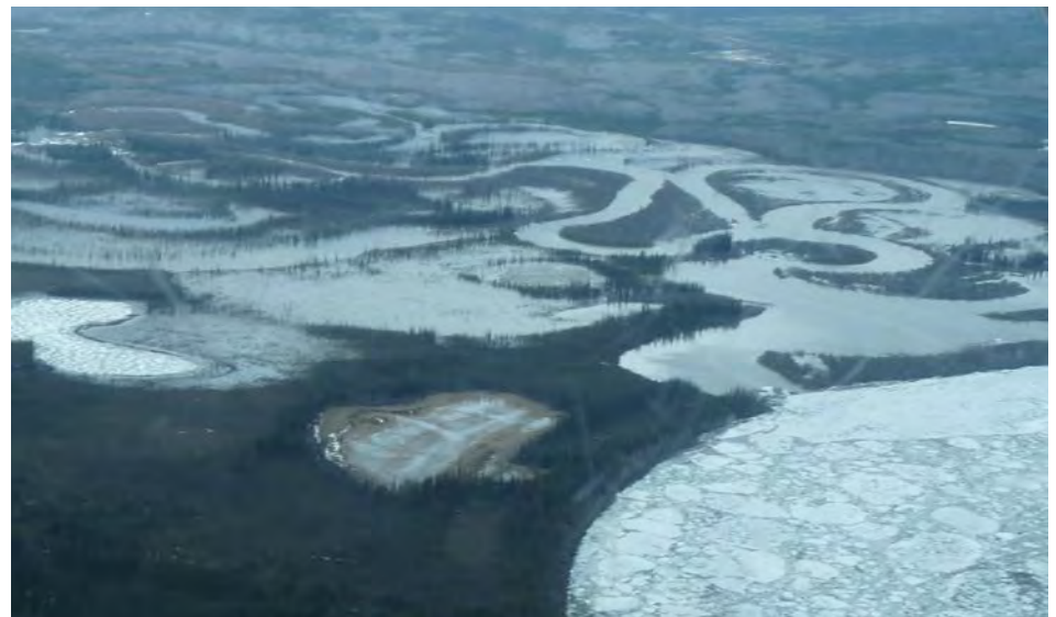
Tributary entering the Yukon graphically displays backwater flooding as the high levels on the Yukon prevent water in Hess Creek near Rampart from entering the Yukon, causing upstream flooding, May 10, 2009. Photo courtesy of Scott Lindsey, National Weather Service
