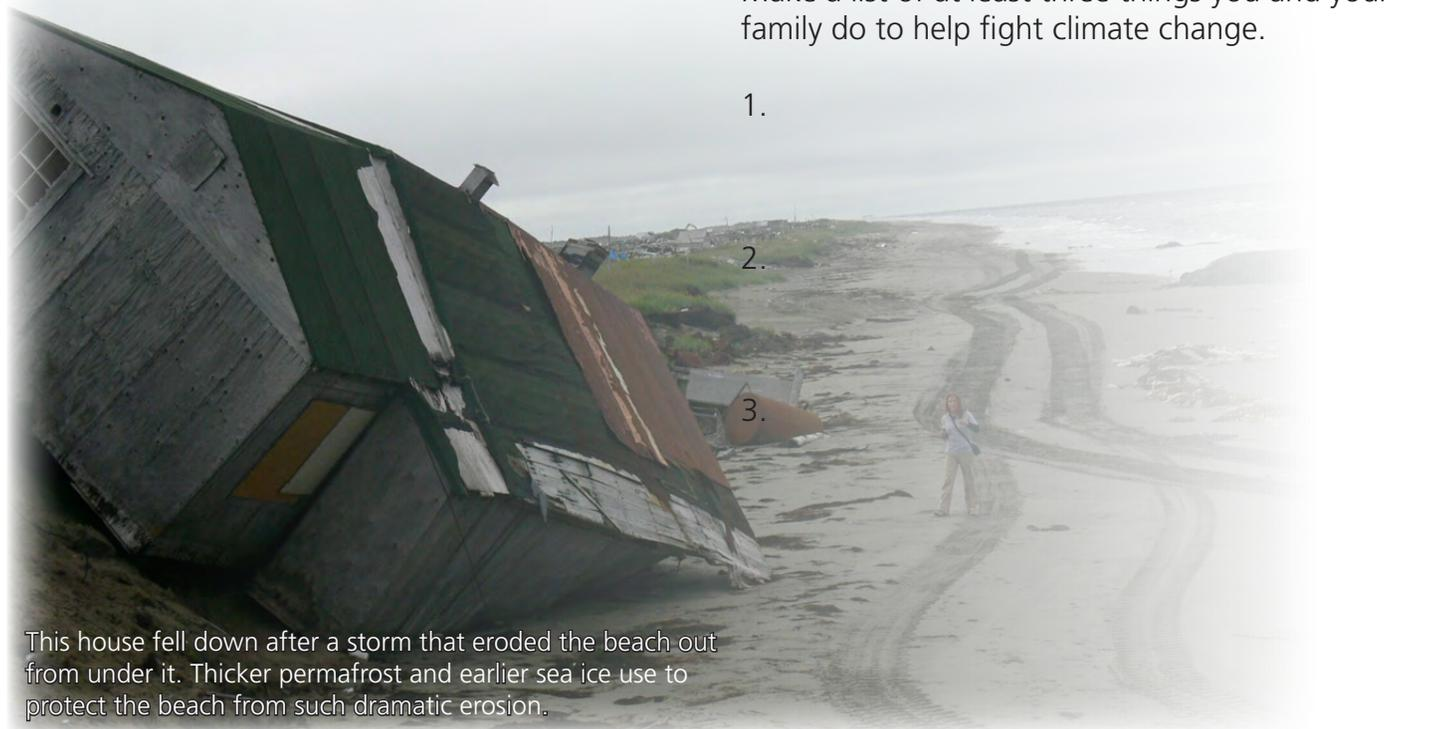
This house fell down after a storm that eroded the beach out from under it. Thicker permafrost and earlier sea ice use to protect the beach from such dramatic erosion.
