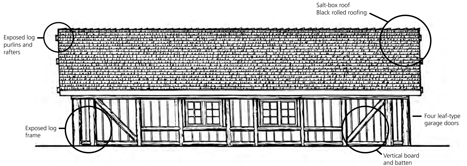
Figure 46. Building 103, South Elevation, Historic American Building Survey, National Park Service, W. Vandeventer and Dave Snow, 1986 (Alaska Regional Office Files)
