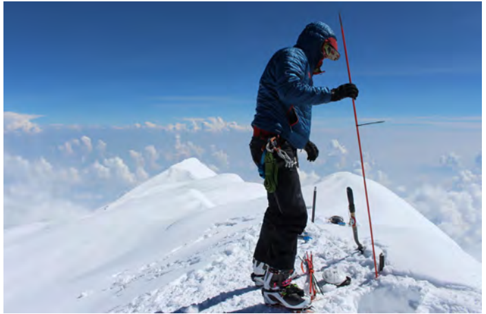
GPS survey conducted in May 2015 on Denali's South Peak to update height of the mountain.
