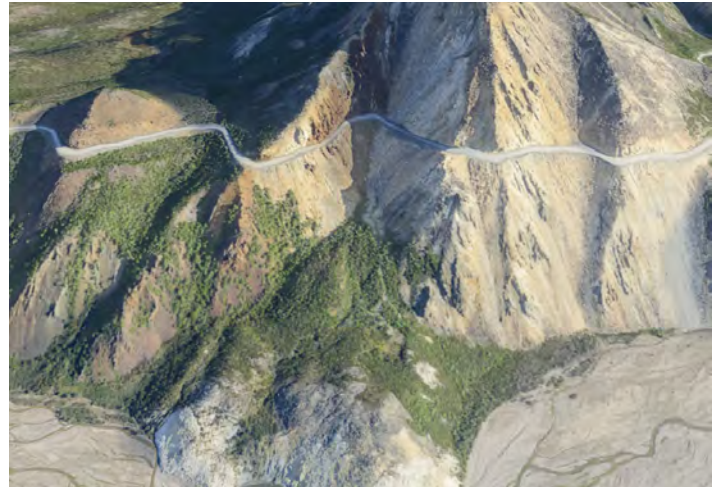
The Pretty Rocks debris slide is shown as an example of composite imagery created through digital aerial photogrammetry.
