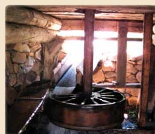
Small mills with horizontal water wheels ground wheat, corn, and chile for villages along the Camino Real. The mill here is perhaps the only one of its type still working in New Mexico.
