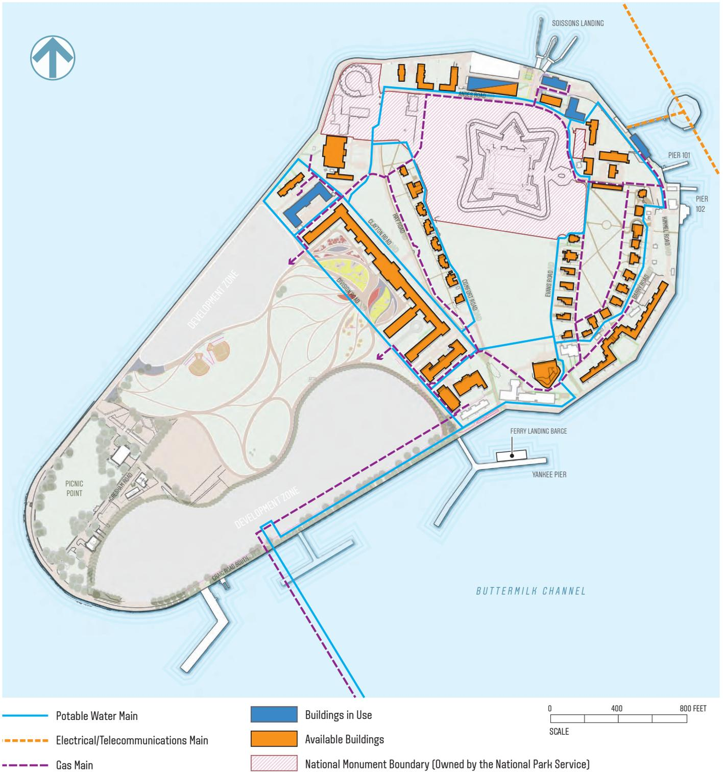
NOTE: \*New electrical feeders and new fiber optic lines will be installed through the Brooklyn-Battery Tunnel. The Trust will replace critical transformers, conduits, and feeders in the Historic District as needed.
