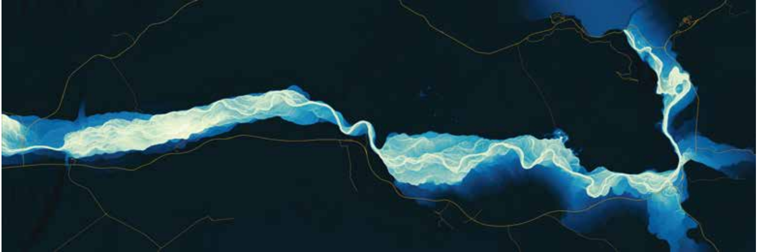
Map of the Snake River, from the outlet of Jackson Lake to Moose, made using Lidar imagery to show elevation changes in the river bottom. This highly accurate mapping tool reveals the history of braided channels. It is featured in part on the back cover. Created by Madeline Grubb, NPS Academy- GIS and Geoscience Member.
