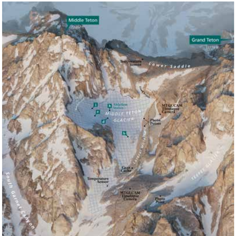
Middle Teton Glacier survey sites and ablation stake placement locations that measure the amount of ice melt or snow remaining and glacier velocity.
