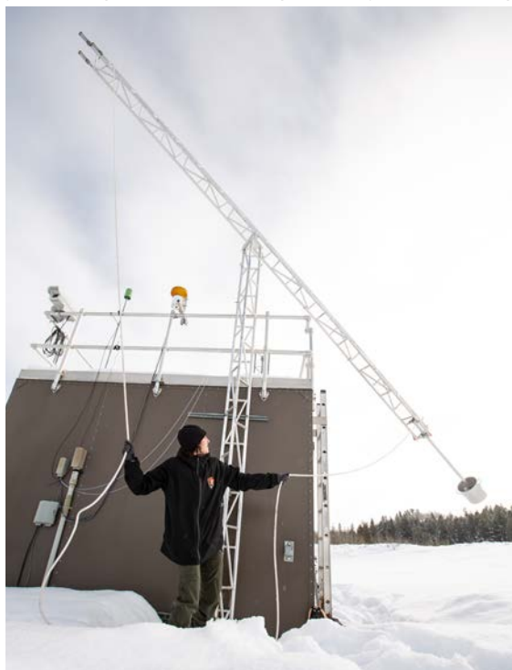
Park staff maintain the air quality station replacing parts like the particulate filter on the ozone measuring instrument.
