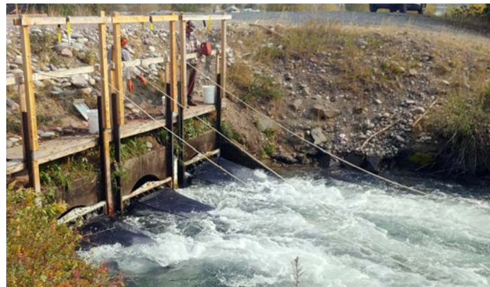
Biologists place nets on the Granite Ditch headgates to capture, count, and measure fish being swept into the irrigation diversion.
