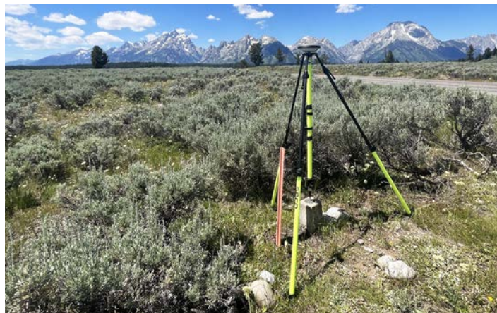
Ben uses satellite positioning tools and precise measurements to update survey benchmark information.
