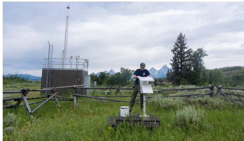
Park scientists swap out the sampling bucket that is part of the National Atmospheric Deposition Program. Collected precipitation samples are sent to a lab for chemical analysis.
