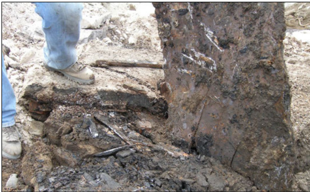
Figure 34. Cork and Stucco Paradise Façade Material (Oriented horizontally with plaster surface on top, and measuring approximately 3m (L) x 1m (W) x 12cm (thick); sample recovered)
