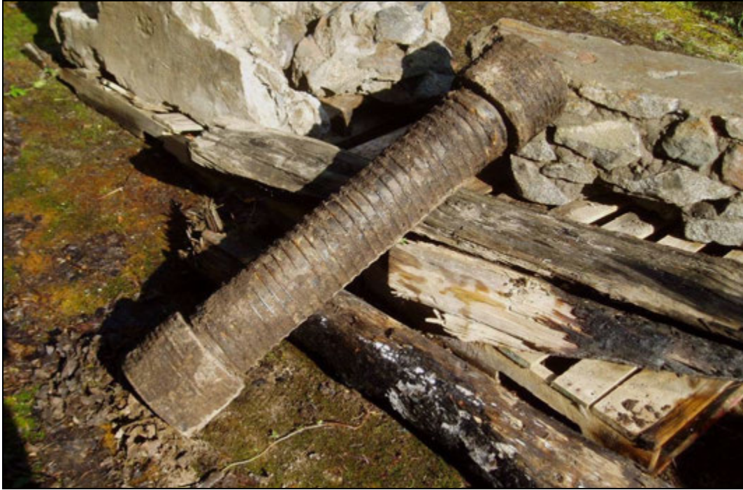
Figure 28. Sample of Recovered Paradise Camp Lodge Structural Elements. Wire wrapped, wood-stave water or sewer pipe at photo center. Charred Alaska yellow cedar decorative building-facing beams, and mortared stem wall sections on palettes.
