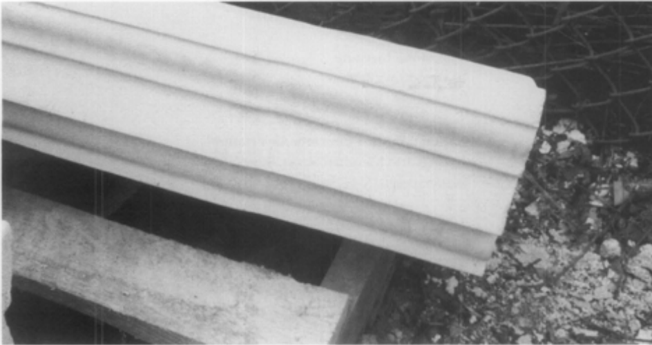
Figure 24. Separation of an interior rubber mold from a plaster mother mold during casting may result in rippling or irregularity of the completed casting.
