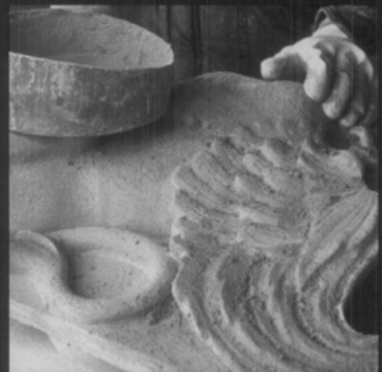
Figure 20. (top) After removal from the mold, new cast stone units are so finished (as shown) to remove surface paste and expose underlying aggregate. (middle) And cast surfaces, such as columns or sculpture, may have numerous air bubbles at the surface. (bottom) The holes on the surface of the casting are filled with a mortar similar to the concrete mix used to cast the element.
