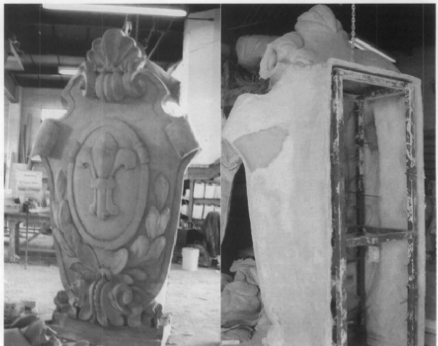
Figure 25. Glass Fiber Reinforced Concrete (GFRC) is sometimes used to replicate deteriorated elements of cast or fine grained natural stone. Because the GFRC element is a rigid, but relatively thin shell, it must be supported and attached with an interior framework of steel. The attachment hardware inside this GFRC cartouche (left) will not be visible when the unit is installed (armature visible at right). Photos: Towne House Restorations, Inc.
