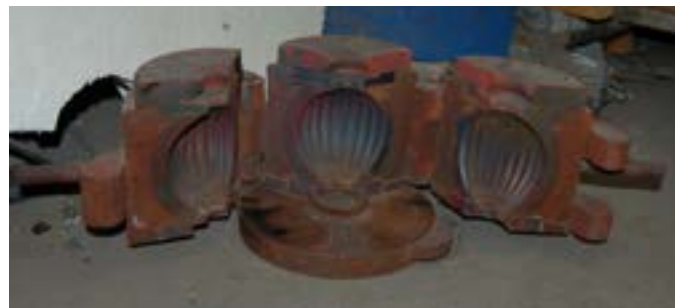
Figure 16. This three-piece vintage mold for a round pleated-glass lightning rod ball is still used to make accurate reproductions today. Photo by author.
