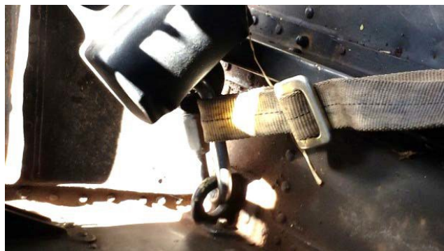
Fig. 3. Example of approved seat belt anchor.
