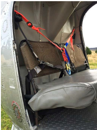
Fig. 2. Example of approved seat belt anchor.
