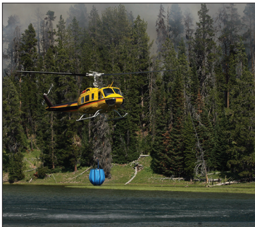
Helicopters are often used in firefighting to cool down a fire with large buckets of water.
