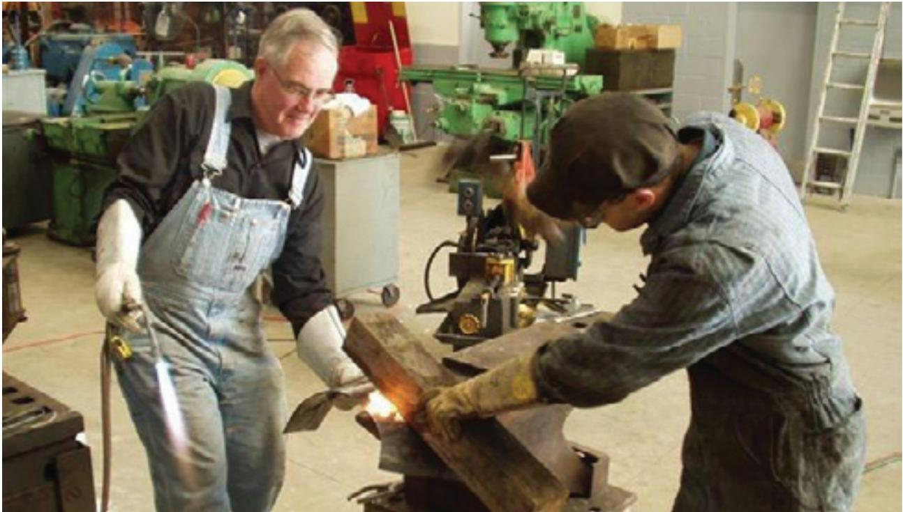
Two B&O Railroad Museum Restoration Shop craftsmen fabricate a piece of the smokestack for the B&O #305 Davis Camel locomotive, one of two surviving "camel" type engines in the world. The restoration of this locomotive, as well as the seven other extremely important steam engines, was needed after the B&O Railroad Museum's roundhouse roof collapse in 2003. Partial funding for the restoration came from the City of Baltimore through the BHAA Small Capital Grant Fund.
