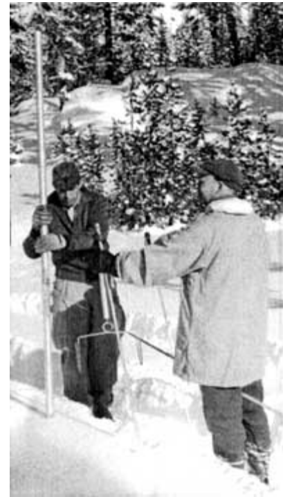
Rangers McLaren and Evans measuring snow pack at Snow Flat at Tioga Pass.
