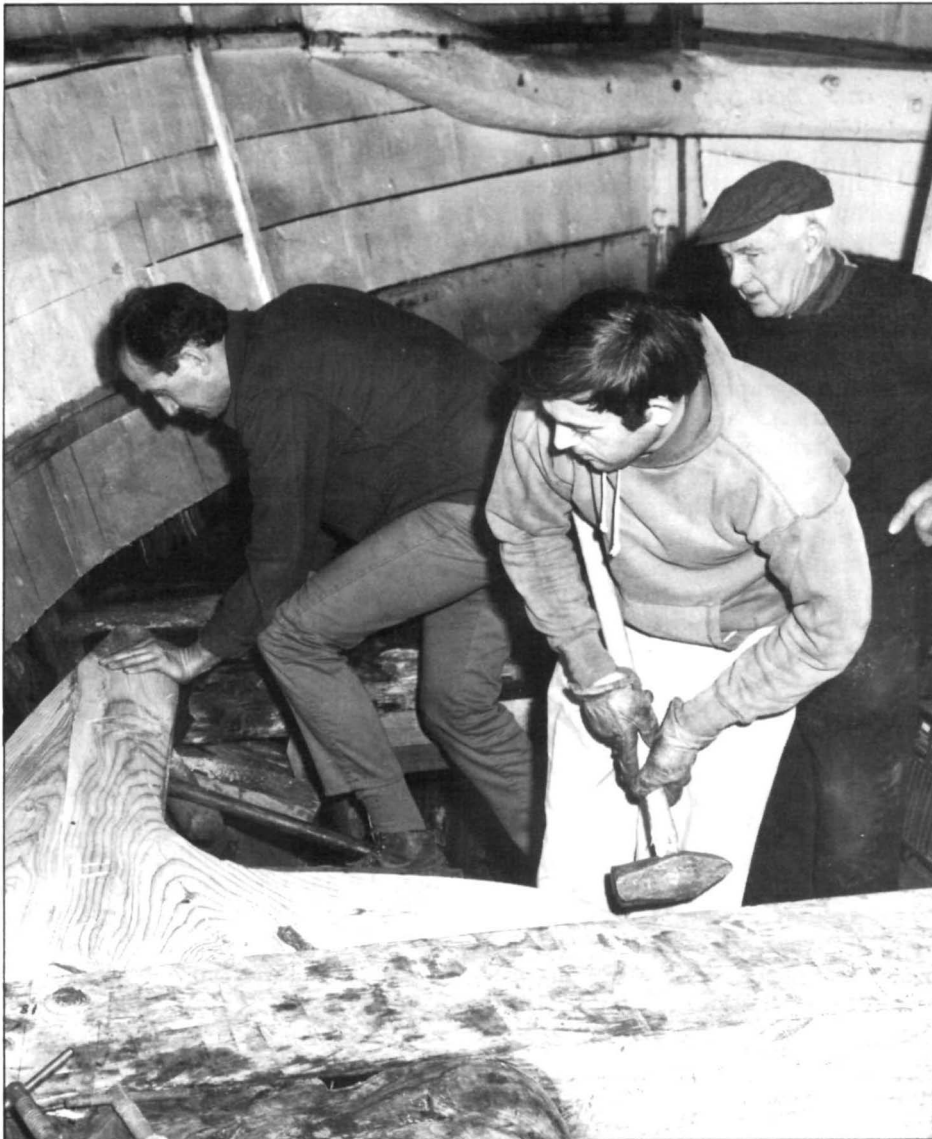
FIGURE 10: An in-kind historic restoration of the whaler Charles W. Morgan at Mystic Seaport Museum. Here shipwrights are driving a drift into a breasthook. (Photo credit: Mary Anne Stets, courtesy Mystic Seaport Museum)
