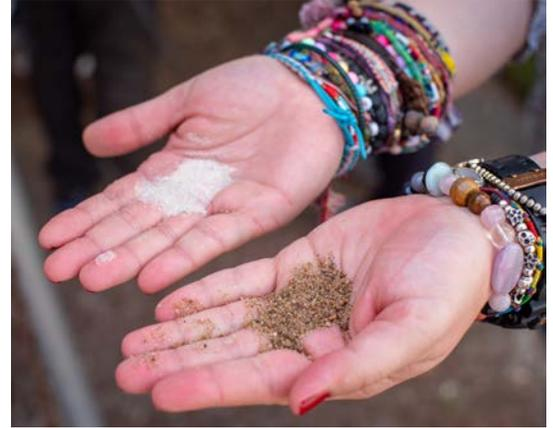
Fine sand was used in plaster coating versus coarse sand was used in repair mortar.
