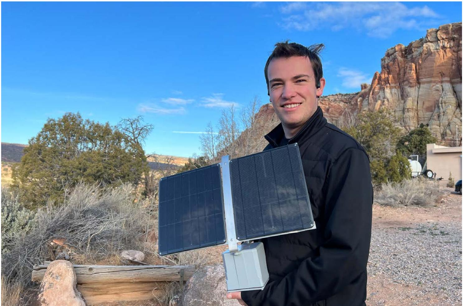
**A student holds a SPARK Beacon that provides the necessary internet connections for media sources in a remote area.**
