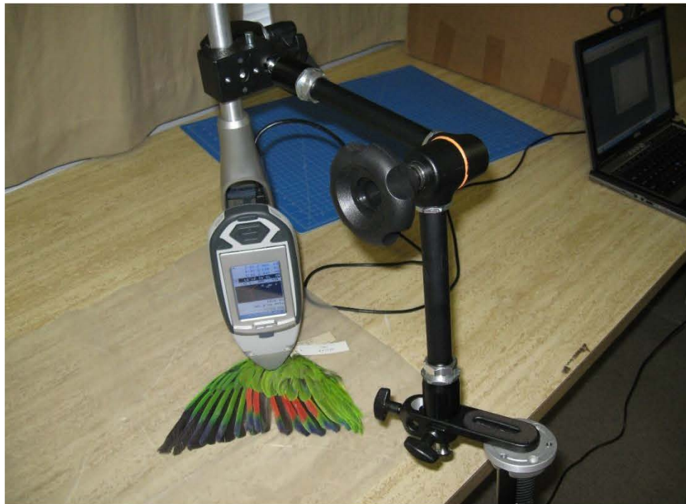
XRF (X-ray florescence) device testing for heavy metal contaminants in bird feathers
