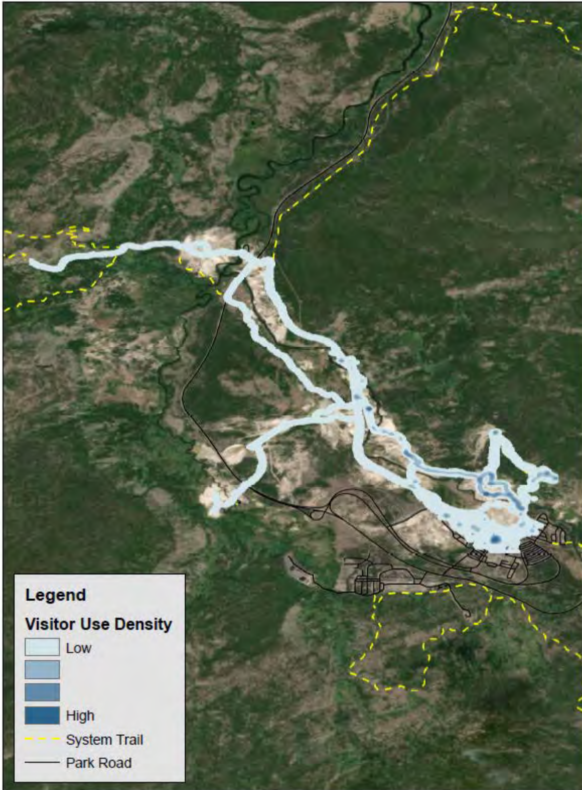
Figure 64. Density of GPS-based tracking points collected from visitors at Old Faithful Geyser Basin. GPS units were handed out between the Visitor Center and Old Faithful Geyser. Low densities are an estimated count 7-96 points per 1 m 2 and high densities are an estimated count of 837-1,888 points per 1 m 2 .
