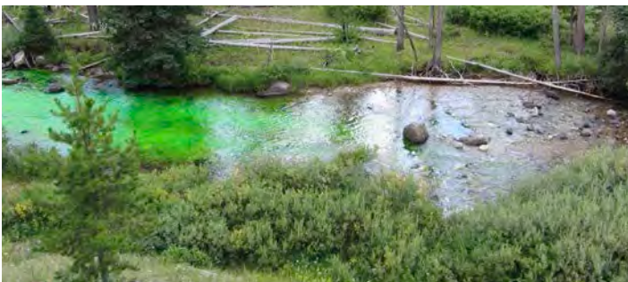
Flow time data is collected by putting biodegradable, fluorescent green dye into the water and following it downstream.
