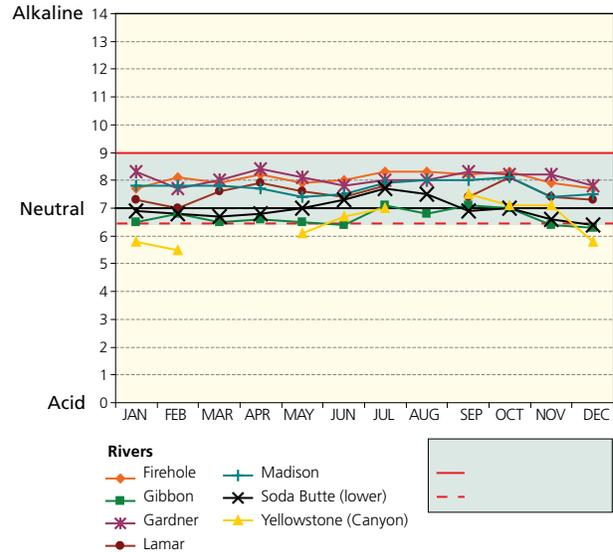
Water quality monitoring data for pH in 2008. The EPA has determined that pH levels from 6.5 to 9.0 are optimum for freshwater aquatic life. Yellowstone waters are sometimes more acidic, especially the Gibbon River, because of geothermal influences.
