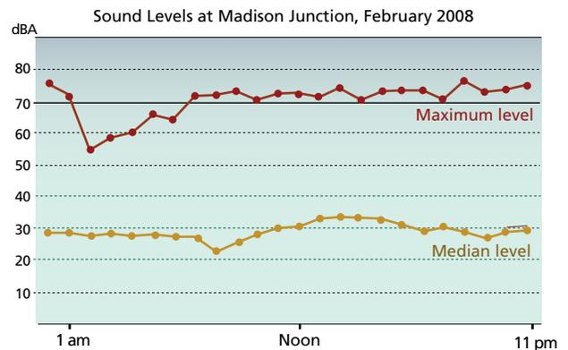
The average and median sound level 100 feet from the road at Madison Junction remained well below the 70 dBA threshold, but the maximum sound level frequently spiked above 70 dBA; 93% of the spikes were from snowcoaches.
